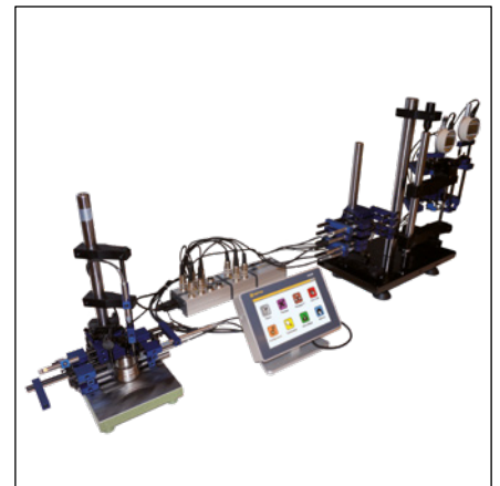
Probes and indicators connection through M-BUS inputs
