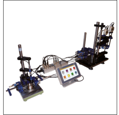
Probes and indicators connection through M-BUS inputs
