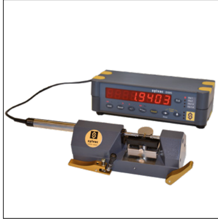
PS15 with connected to a D50S
