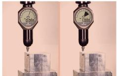
Danger of crash (0 mm till ERR01) When overpassing, the LED warns in red and the black bar builds up clockwise to the right. Shortly before crash (>1 mm), you can see ERR01 on the display..
